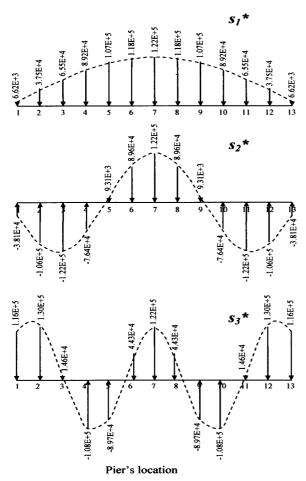
Figure 7. Force Distribution  $s_n^* = m\phi_n$ , n = 1, 2, 3 (at Pier's Top Elevation)
