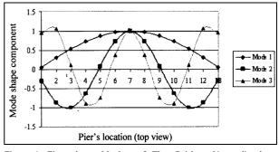
Figure 6. First three Modes of The Bridge, Normalized to Pier's Top of Pier 7
