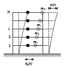
Figure 1. N-DOF System Under Ground Motion
