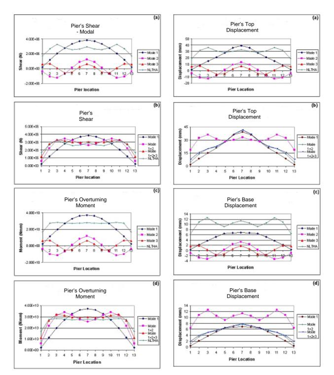
Figure 11. Pier's Shear and Overturning Moment from UMRHA
