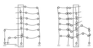
**Figure 11.** Frame 6 Plastic Hinges due to Maximum Considered Earthquake in x-direction
