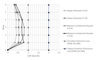
**Figure 7.** Drift Ratios of Hotel X due to Design and Maximum Considered Earthquake Compared to FEMA 356-2000 limits
