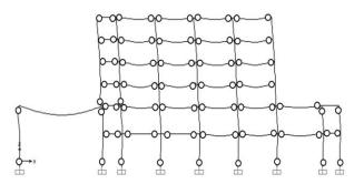
**Figure 10.** Frame 1 Plastic Hinges due to Maximum Considered Earthquake in x-direction
