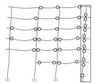
Figure 13. Frame I Plastic Hinges due to Design Earthquake in y-direction
