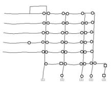
**Figure 14.** Frame D Plastic Hinges due to Maximum Considered Earthquake in y-direction
