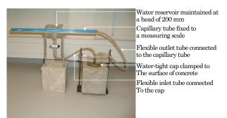
Figure 1. A Typical ISAT Set-up
