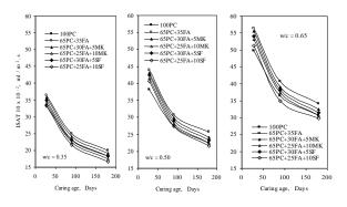
**Figure 5.** ISAT 10 of PC, FA Binary Cement and SF and MK Ternary Cement Concretes at 35% Total Replacement Level and Water/Cement Ratios of 0.35, 0.50 and 0.65
