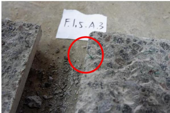
**Figure 6.** The Full-sized Length of Welded Wire Mesh Sticking Out from the Concrete Surface
