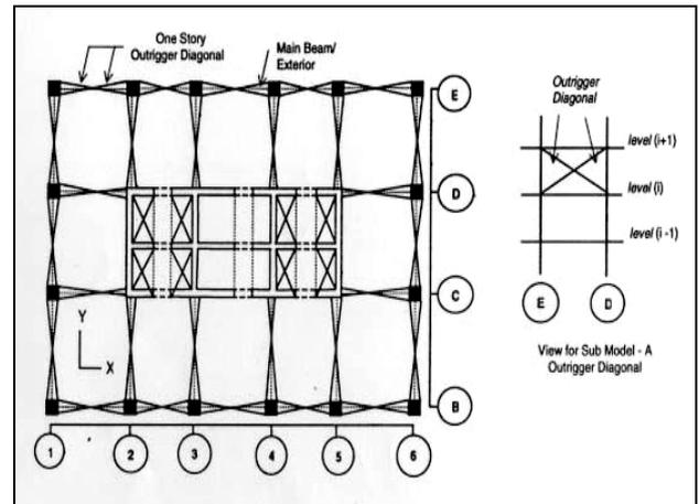
Figure 8. The Structural Model with single or double outrigger diagonal- Model A
