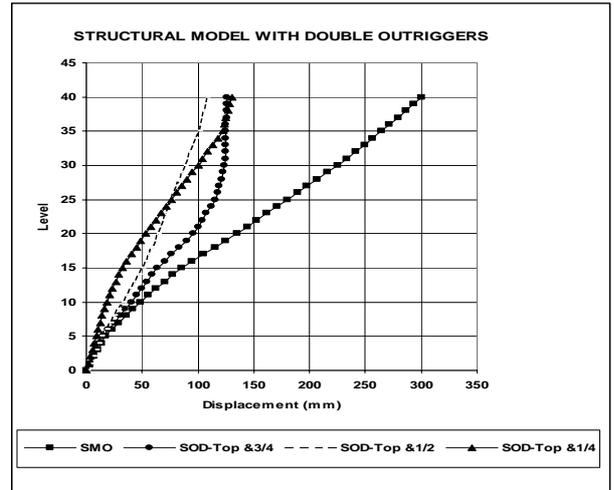
Figure 6. The Lateral Displacement of Structural Model with Double Outrigger
