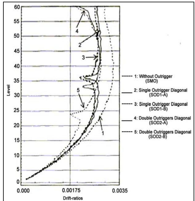
Figure 13. The Inter-storey drift ratio (For optimum location of the outrigger with dynamic analysis).
