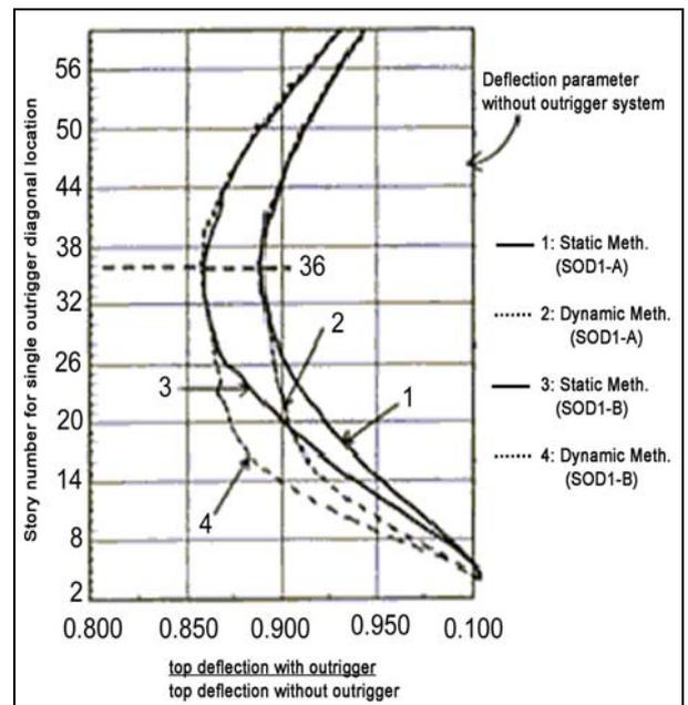
Figure 10. The Optimum Location for Structural Model with single Outrigger.
