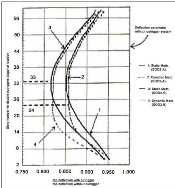
Figure 11. The Optimum Location for Structural Model with double outrigger.
