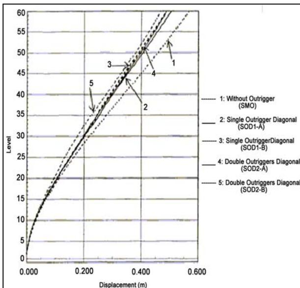
Figure 12. The Lateral Displacement ratio (For optimum location of the outrigger diagonal with dynamic analysis)
