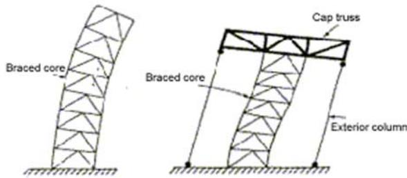
Figure 2. The Braced Core and The Braced Core, Exterior Column, and Cap Truss [1]
