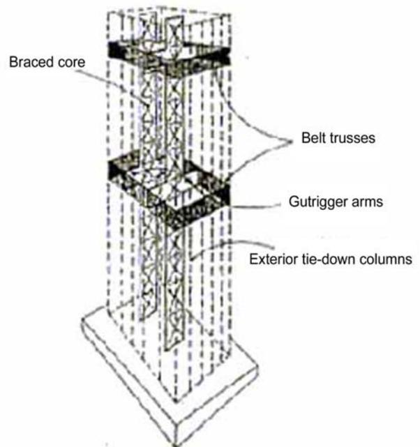
Figure 1. The belt truss system [4]
