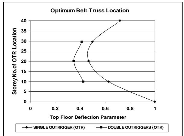
Figure 7. The Optimum Belt Truss Location
