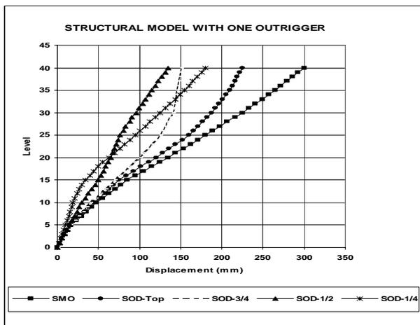
Figure 5. The Lateral Displacement of Structural Model with One Outrigger.
