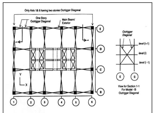
Figure 9. The Structural Model with single or double outrigger diagonal- Model B
