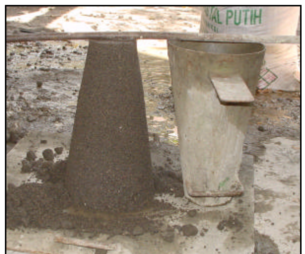
Gambar 2. Hasil Test Slump Benda Uji
