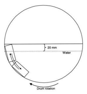
Figure 5. Rectangular specimens in the slake-durability drum.
