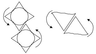
Figure 6. Irregular rock lumps in slake-durability tests of soft rocks.
