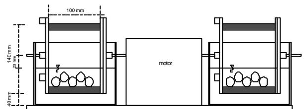
Figure 1. The slake-durability test apparatus.
