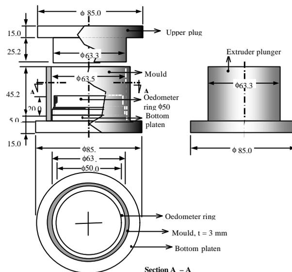
Figure 3. Static compaction mould for swelling specimens.
