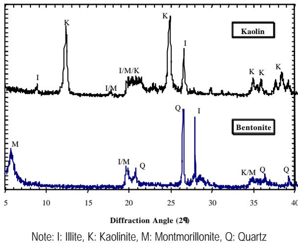
Figure 4. X-Ray diffraction of kaolin and bentonite soils.
