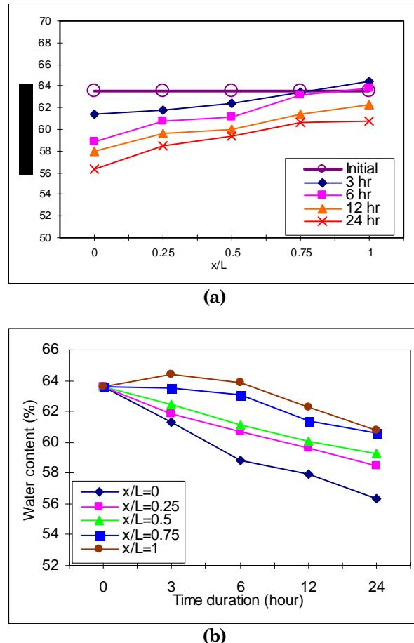
Figure 4. The water content variation on the location of anode (a) and the time duration (b)
