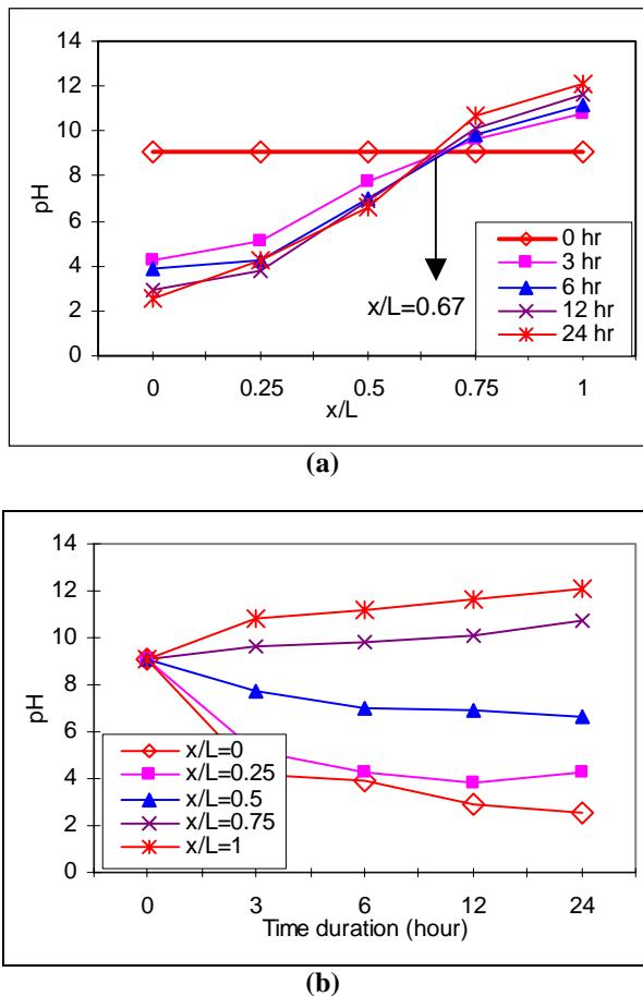
Figure 5. The pH Value Variation on Location of Anode (a) and Time Duration (b)
