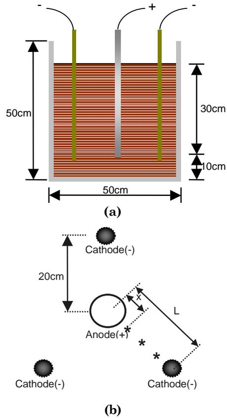
Figure 2. Model (a) and Configuration (b) of The Electrodes in The Soil Sample
