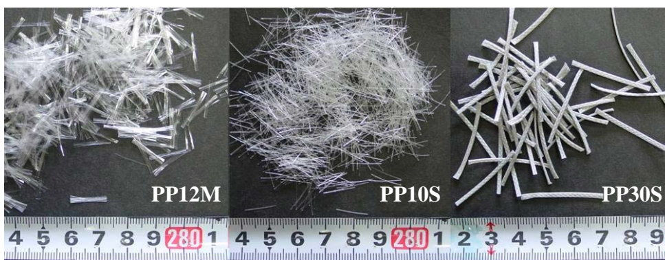
Fig. 2. Three types of polypropylene fiber used and their designations
