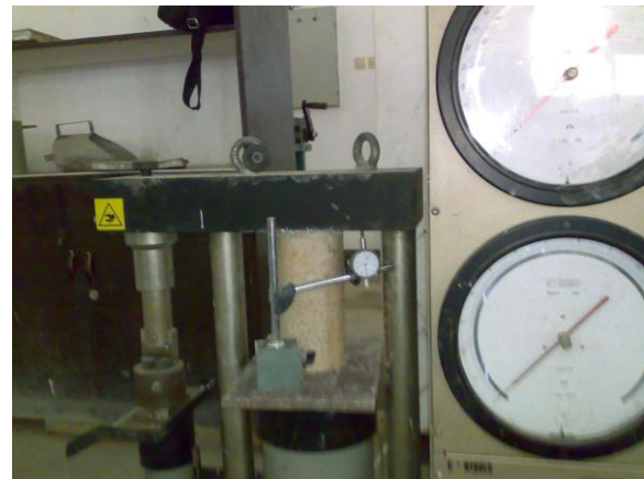
Figure 2. Unconfined compression test on plaster-pumice mixed materials
