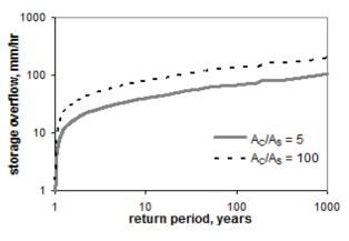
Figure 2. Flood Frequency Curve of Storage Overflow
