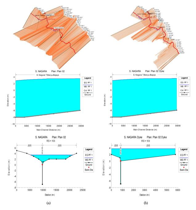
**Figure 4.** River Geometries (top figures), Water Surface for Long Profiles (middle figures) and Cross Sections (bottom figures) in the Simulation at Existing Condition or without Dyke (a) and with Dyke (b)
