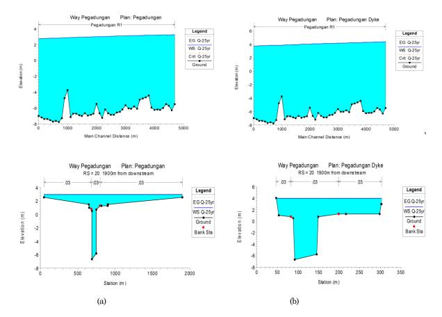
**Figure 3.** Water Surface for Long Profiles (top figures) and Cross Sections (bottom figures) in the Simulation at Existing Condition or without Dyke (a) and with Dyke (b)
