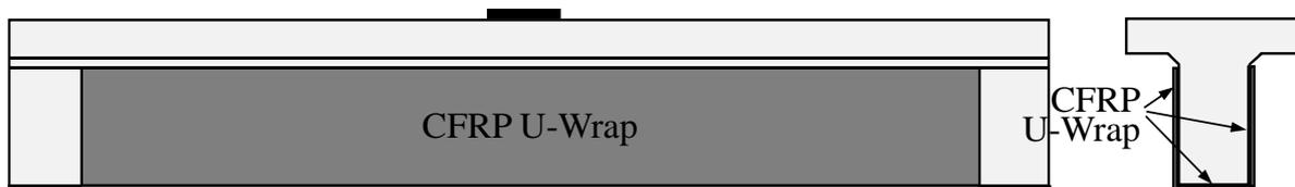
**Figure 2.** Layout of CFRP Strengthening for Beam LB1U
