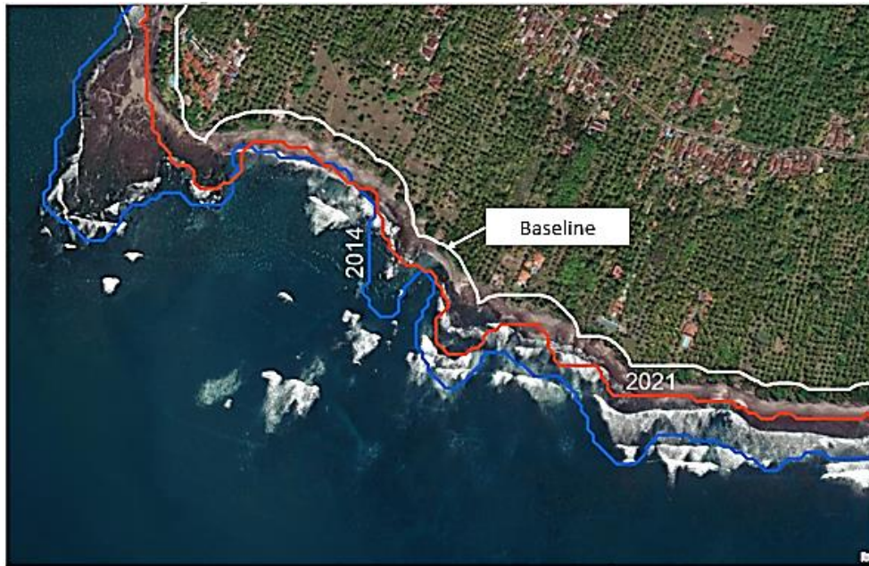
Figure 2. Example of a Baseline (Reference Line) Making Process from Coastline Data for 2014 and 2021
