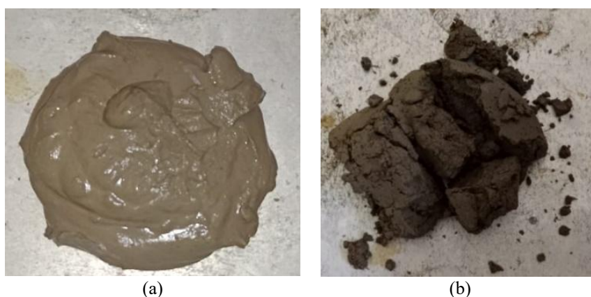
Figure 2. Consistency of Clay Shale with a Mixture of a) SCU-CP Solution, b) PCP Solution
