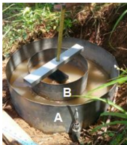
Figure 3. Double Ring Infiltrometer Set Up in the Field
