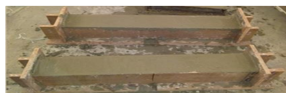
(b) BFRC Beams
