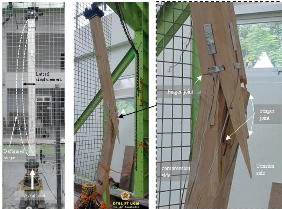
Figure 5. The Buckling Failure of the Specimen
