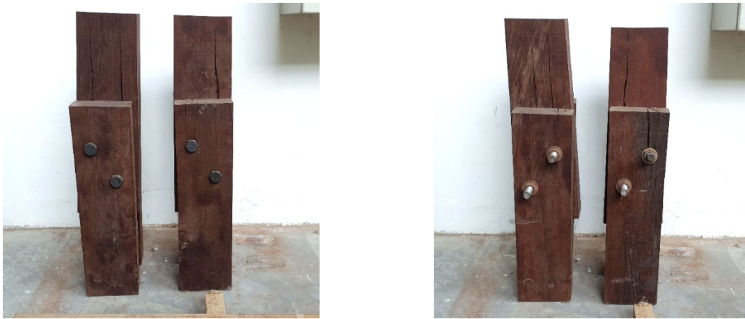
Figure 12. Wood Failure from the Side
