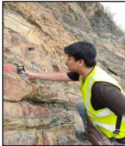
Figure 8. Measurement of Dip Angle and Dip Direction by using Geological Compass
