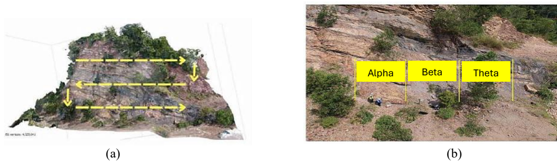
Figure 3. Photogrammetry Survey: (a) Drone Flight Path, (b) Three Divided Zones
