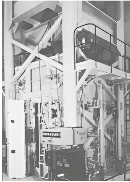
Figure 1. Column Test Furnace [25]
